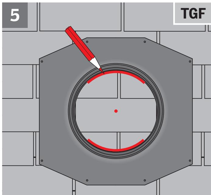
**ENGLISH:** Locate the nail indicating the center of the sun tunnel on the roof and use the flashing to mark top and bottom of the rough opening.
