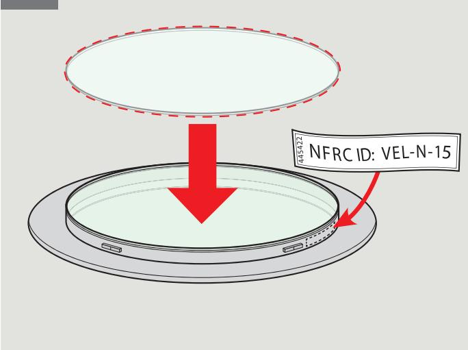
**ENGLISH:** Install the secondary diffuser disc onto the primary diffuser and apply the enclosed NFRC label to the back of the diffuser as shown.
