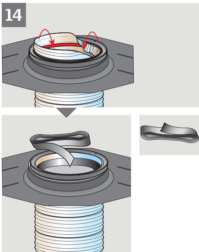
**ENGLISH:** Fold the end of the tunnel over the locking snap ring and secure the loose edge of the tunnel with tape provided.
