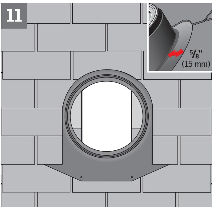
**ENGLISH:** Reinstall roofing material over the flange. Leave a  $5/8"$  (15 mm) channel for water to run off.
