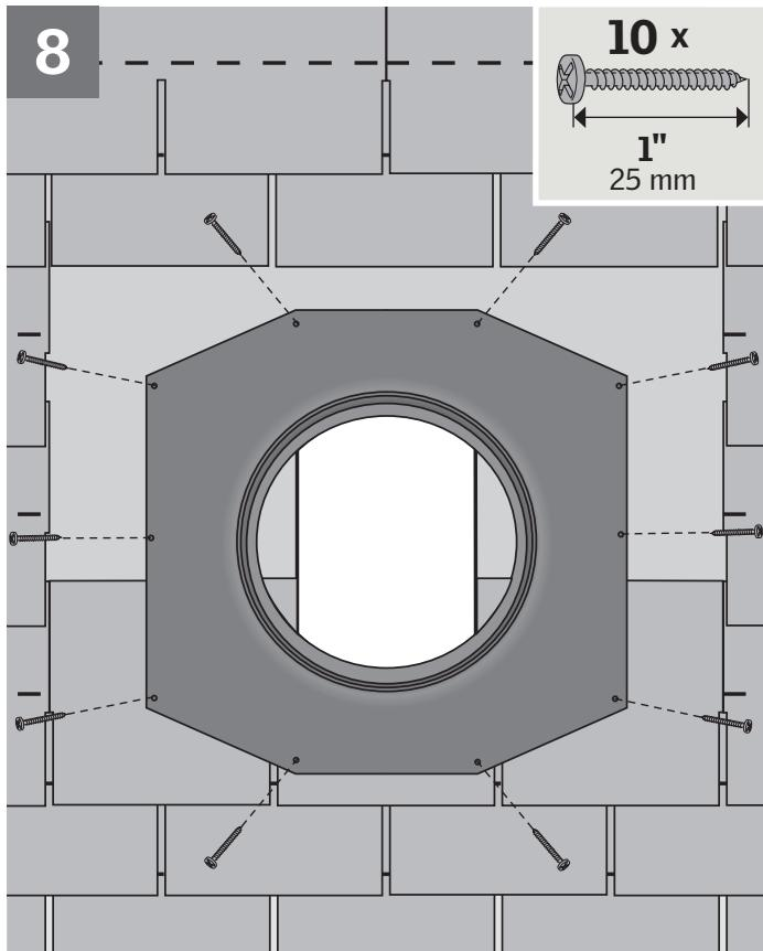
**ENGLISH:** Center the flashing over the rough opening and secure the flange with ten of the provided 1" (25 mm) screws in all the pre-punched holes along the edges.
