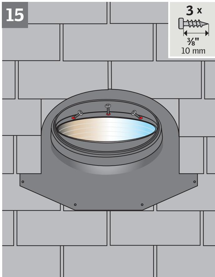
**ENGLISH:** Seat the pivot ring with the tunnel assembly into the flashing. Secure the pivot ring with screws if needed.
