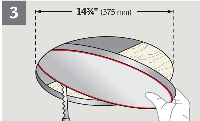
**ENGLISH:** From the inside, locate the nail indicating the center of the sun tunnel in the ceiling, mark circle and cut rough opening in the ceiling as shown.
