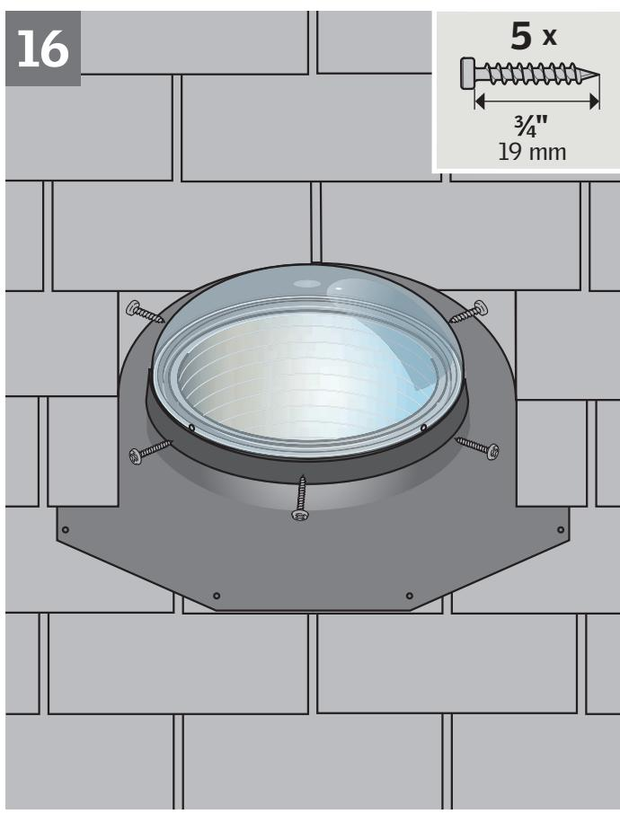
**ENGLISH:** Align holes; install and secure the dome with the  $\frac{3}{4}$ " (19 mm) screws provided. Do not overtighten the screws.
