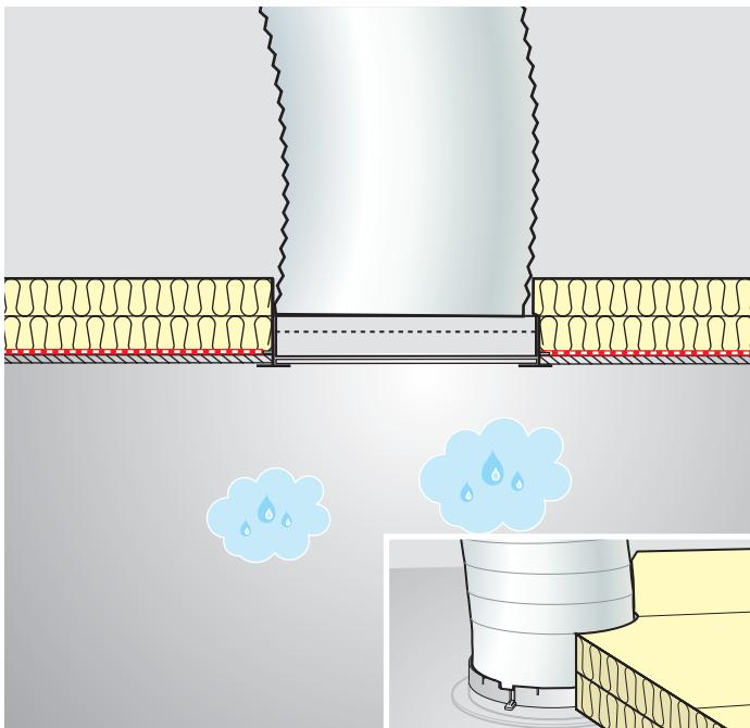
**ENGLISH:** If vapor barrier is installed, insure a tight joint between the ceiling ring and the vapor barrier. Reposition the insulation material around the tunnel.
