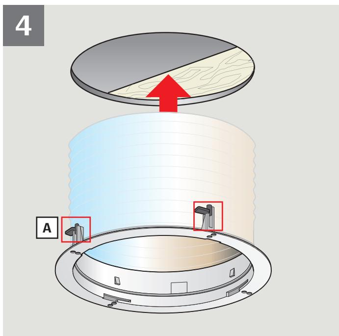
**ENGLISH:** Tip the plastic pins down into hidden position **A**. Insert the ceiling ring assembly. Avoid distortion of the ceiling ring causing the diffuser not to fit smoothly **B**.
