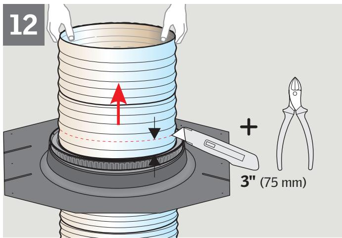
**ENGLISH:** Pull the flexible tunnel section tight through the flashing and pivot ring and cut flexible tunnel to length as shown.
