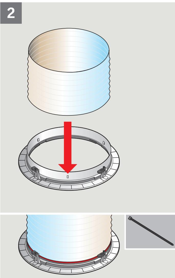
**ENGLISH:** Pull the flexible tunnel section over the ceiling ring. Secure with flexible plastic tie.
