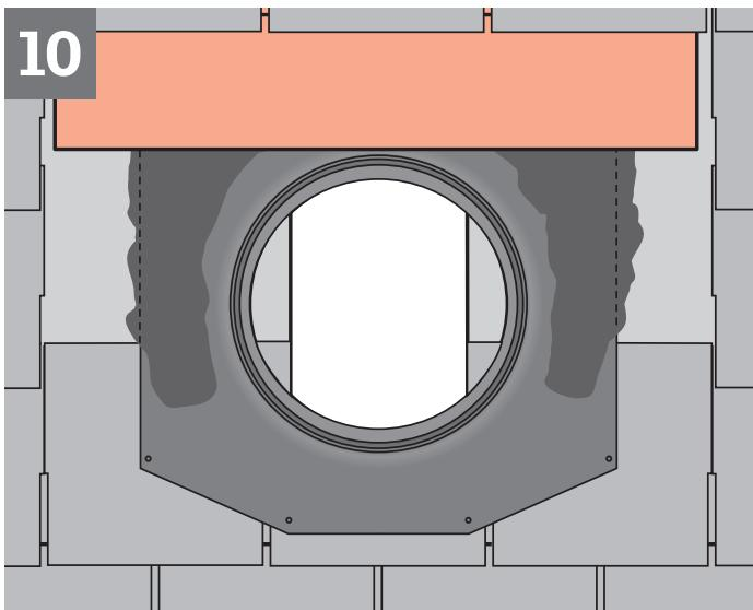
**ENGLISH:** Overlap the top of the flange with underlayment to allow for proper drainage.
